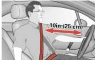
**⚠ WARNING:** The distance from the center of your breastbone to the center of the airbag cover on the steering wheel or instrument panel must be at least 10 inches (25 cm) or more.
