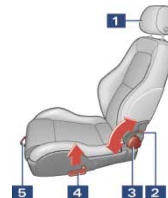
**⚠ WARNING:** Front seat passengers must never ride in a moving vehicle with the seatback reclined. The risk of personal injury increases with increasing rearward angle of the seatback. Safety belts only offer protection when the seatback is upright and belts are properly positioned on the body. Adjust your seats only when the vehicle is at a complete standstill.
